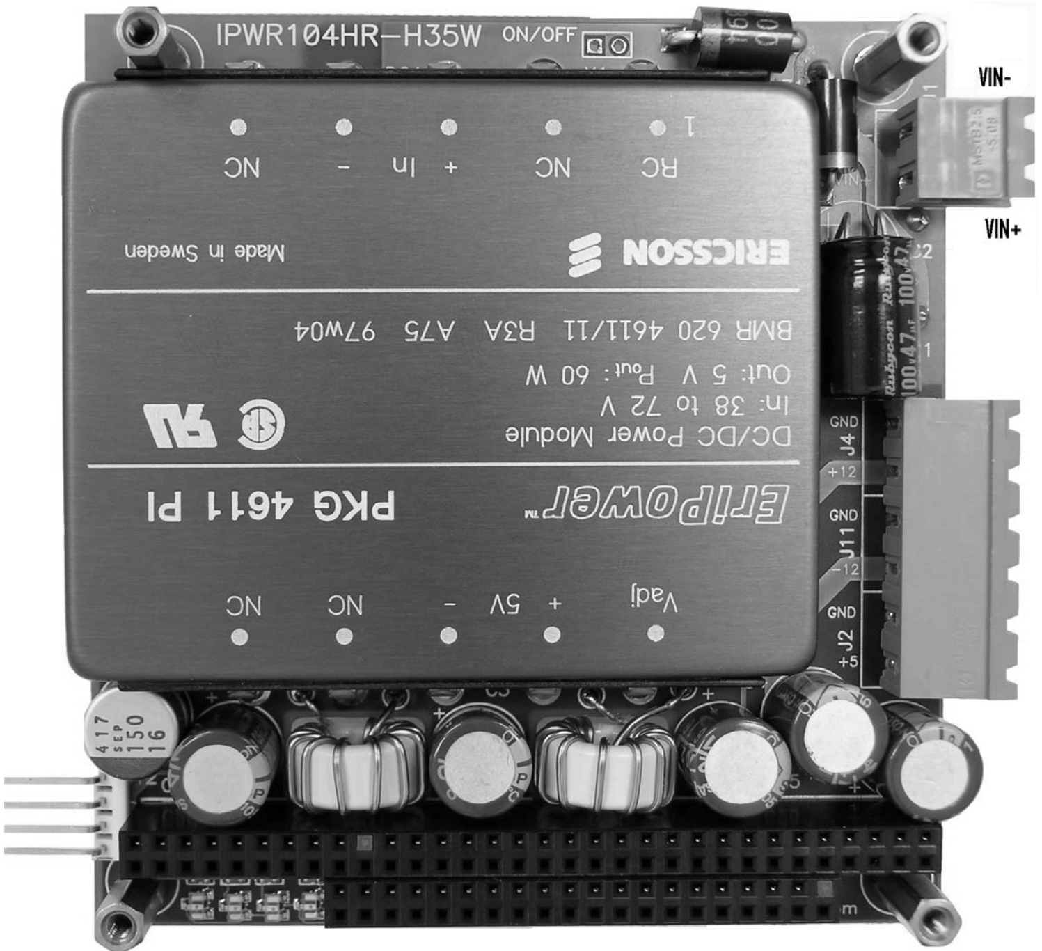
Fig. 2-2 IPWR104HR-H35W shown power supply power connections
