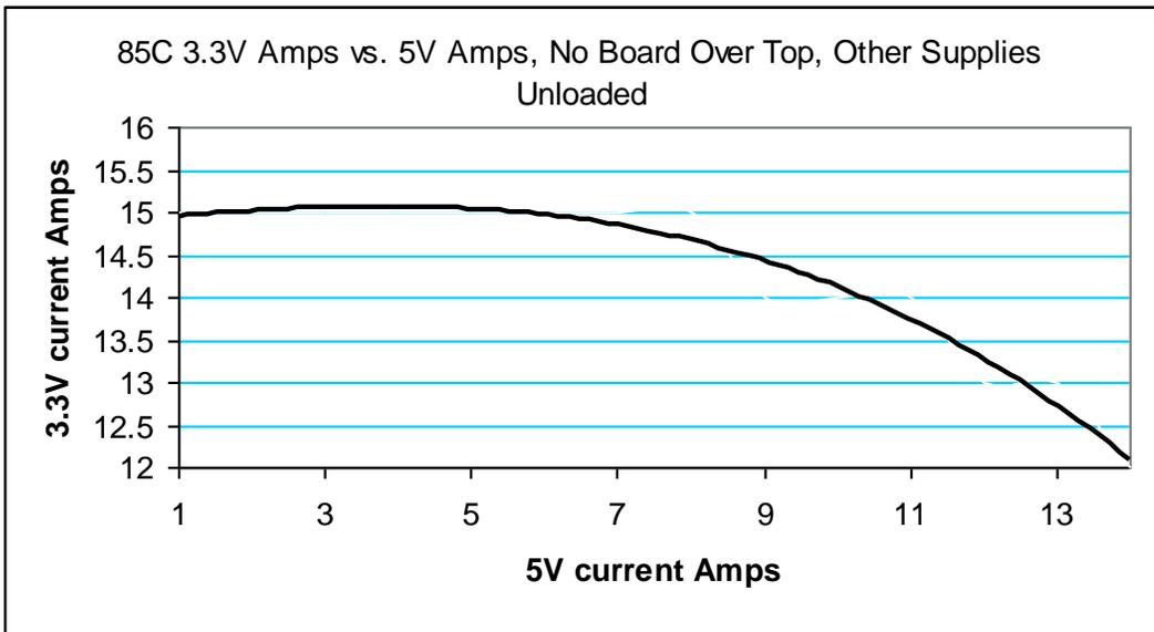
The above graph describes how the 5V and the 3.3V converters cross heat each other at 85C with 44'/min. airflow and no constriction. All other supplies at zero load.
