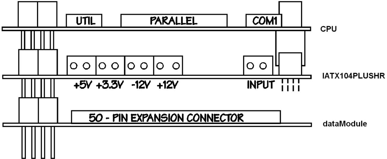
**Figure 1: IATX104PLUSHR powering an RTD PC/104+ cpuModule stack**
