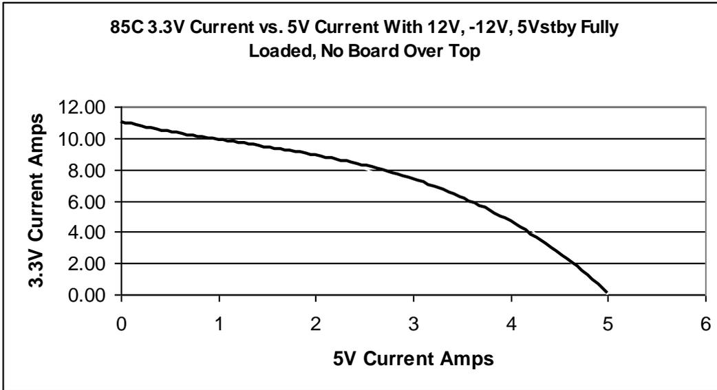
The above graph describes how the 5V and the 3.3V converters cross heat each other at 85C with +- 12V, and 5Vstby fully loaded, 44'/min. airflow and no board over top blocking airflow.
