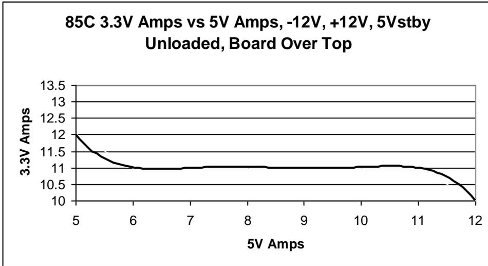
The above graph describes how the 5V and the 3.3V converters cross heat each other at 85C with 44'/min. airflow and a constricting board over top. **All other supplies are fully loaded.**
